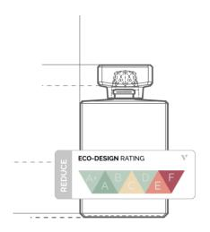
With Glass Score, Verescence offers its customers the ability to evaluate the level of weight reduction of their products, without the influence of the container size. The rating system assigns a score ranging from A+ (the most lightweight) to F for each bottle, enabling brands to compare their products on a universal scale and develop new glass weight-reduction projects.
